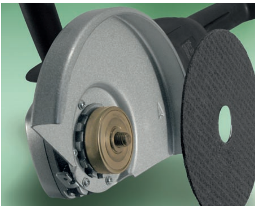
Meets the strict EU limits for the vibration loads of electric power tools: The Autobalancer makes angle grinders more ergonomic
