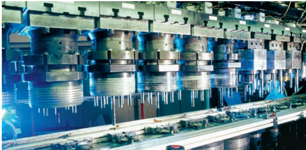
Multiple die press: Highly-developed, deep drawing technology enables economical production of bearing components manufactured by forming methods
