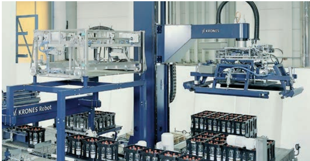
INA linear recirculating roller bearing and guideway assemblies in a packing and palletizing robot mean that the required precision at high loads as well as long-term process reliability are ensured for the machine manufacturer (Photo: KRONES)
