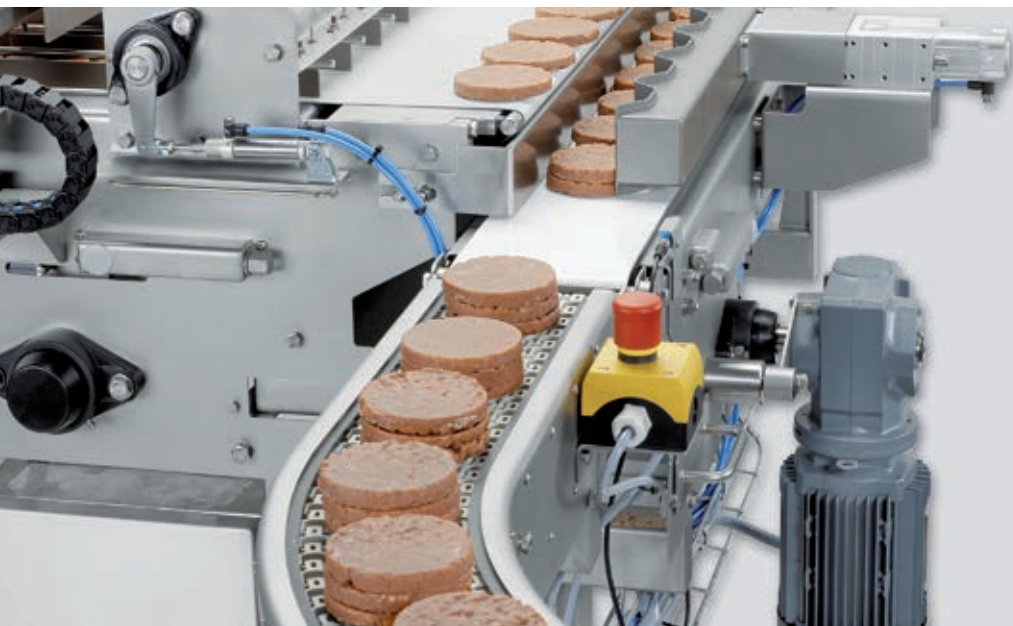
Safe for use with foodstuffs and protected against corrosion: Plastic flanged housings in a waffle conveyor belt system (photo from TMF Belting Systems B.V.).
