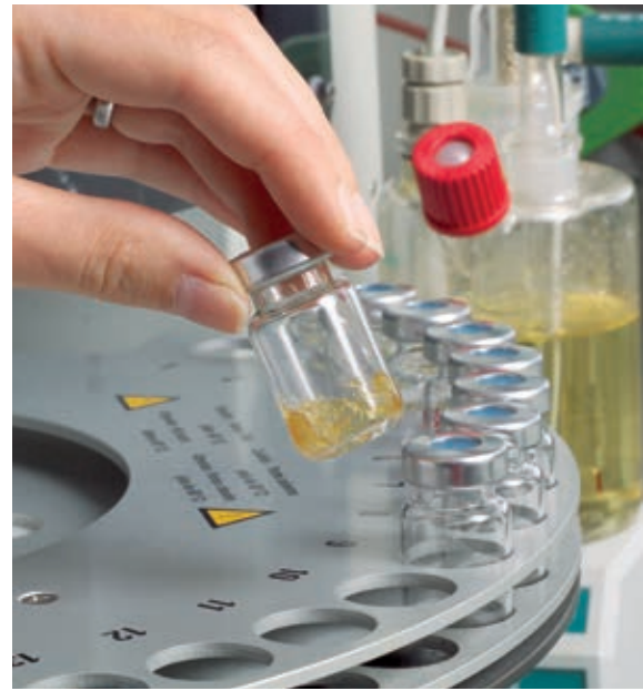
Testing in our in-house lab: Analysis of lubricants for water content
