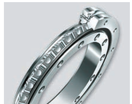
Save on one bearing position: INA crossed roller bearings XSU support radial and axial loads, tilting moments as well as any combination of loads
