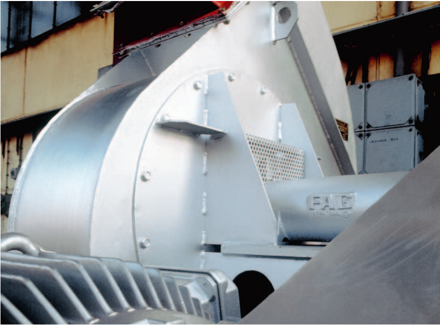
Radial fan with bearing unit VRE
