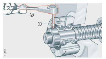
① Set screw ② Tightening torque M<sub>m</sub>
