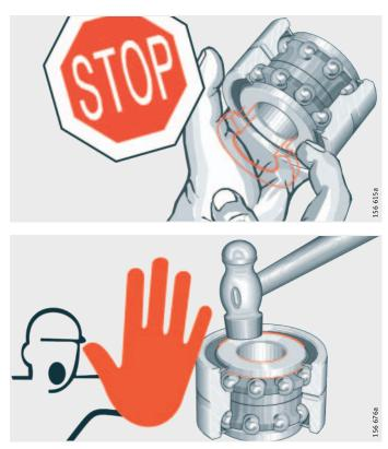
*Figure 5* Do not remove the inner ring halves
