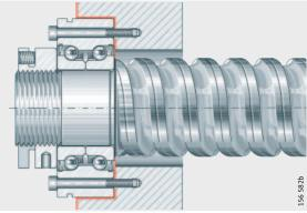
Figure 1 Outer ring screw mounted on flat adjacent construction
