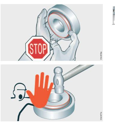
*Figure 5* Do not remove the inner ring
