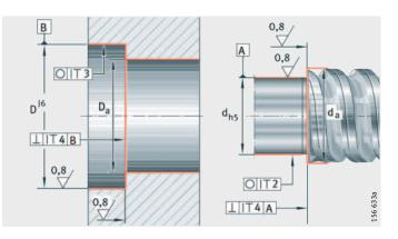
*Figure 2* Design of adjacent construction
