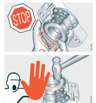
*Figure 5* Do not remove the inner ring halves
