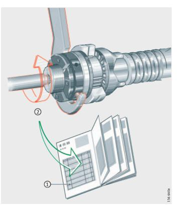
① TPI 123 ② Tightening torque M<sub>A</sub>
