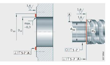
Figure 2 Design of adjacent construction
