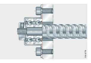
Figure 1 Unit screw mounted on flat adjacent construction
