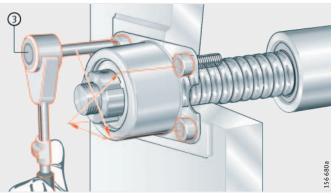
Angular contact ball bearing unit
