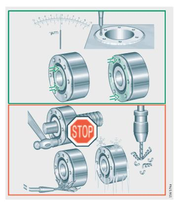
Figure 9 General safety and operating guidelines Fitting of double row axial angular contact ball bearings for screw mounting Series ZKLF, ZKLF..-PE, ZKLF..-2AP
