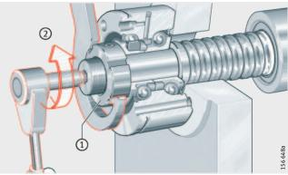
(1) Precision locknut (2) Tightening torque M<sub>A</sub>
