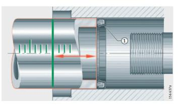
① Rotary shaft seal
