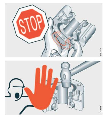
*Figure 7* Do not remove the inner ring halves
