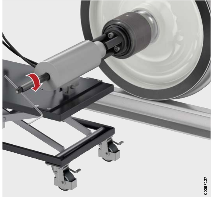
Figure 5 Screwing the spindle into the guide bush
