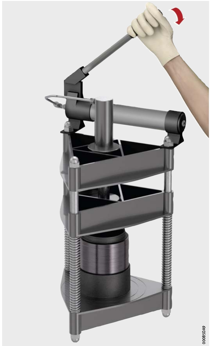
Figure 14 Inserting and aligning the bearing in the press; activating the press
