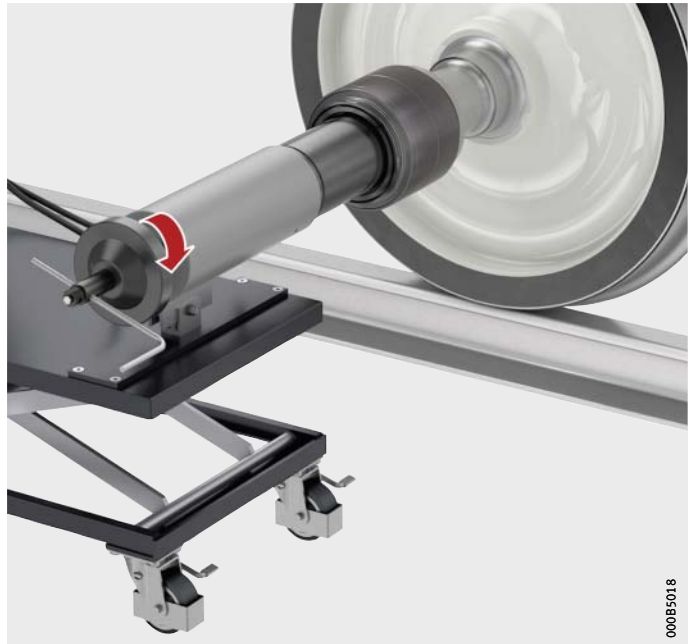
Figure 6 Screwing the spindle into the guide bush
