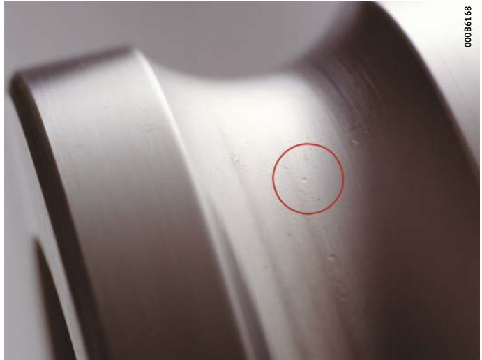
Figure 4 Raceway indentations due to contamination
