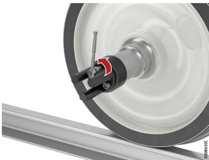
Figure 7 Unscrewing the guide bush
