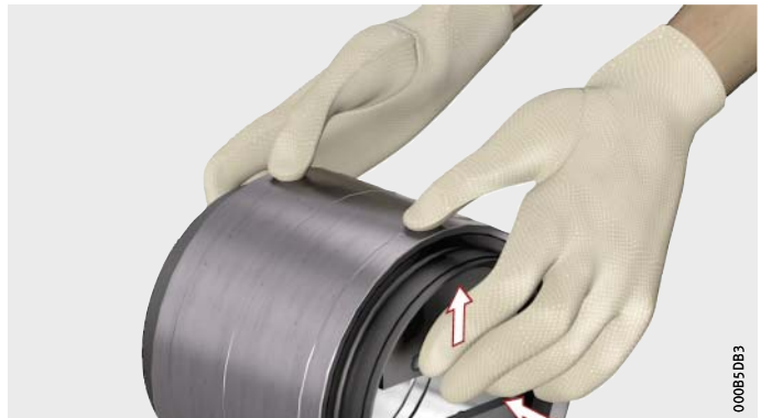
Figure 10 Inserting the press-out segments
