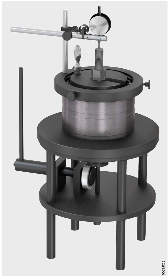
Figure 11 Locating ring with dial gauge
