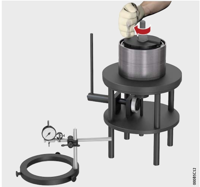
Figure 10 Rotating the outer ring
