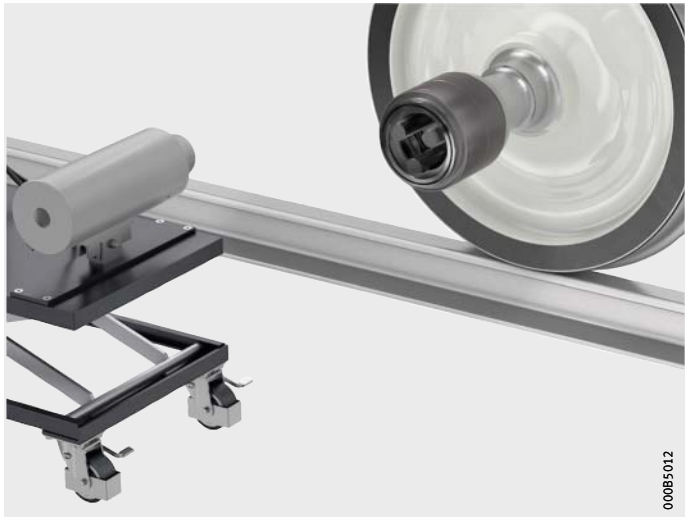
Figure 3 Moving the hydraulic unit into place
