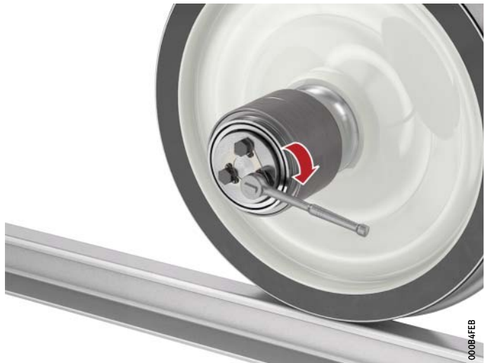
Figure 9 Tightening the end cap screws
