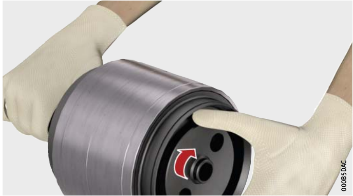
Figure 12 Axially tensioning the punch and segments
