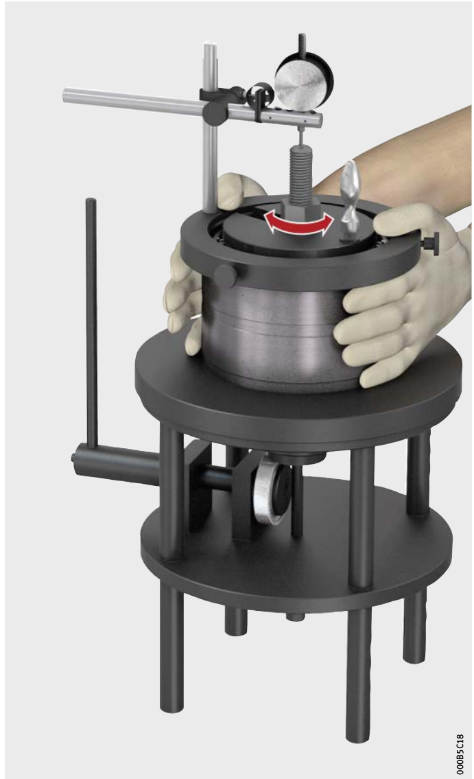
Figure 12 Rotating the outer ring
