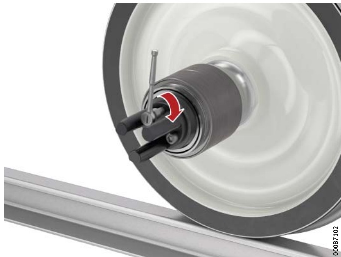
Figure 3 Screwing on the guide bush
