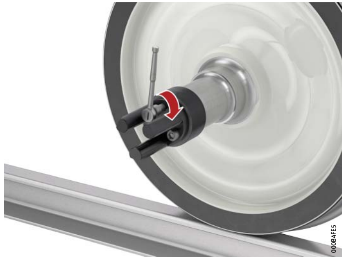
Figure 1 Screwing the guide bush onto the shaft journal
