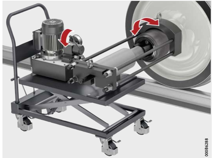
Figure 6 Extractor shoe in contact with shaft
