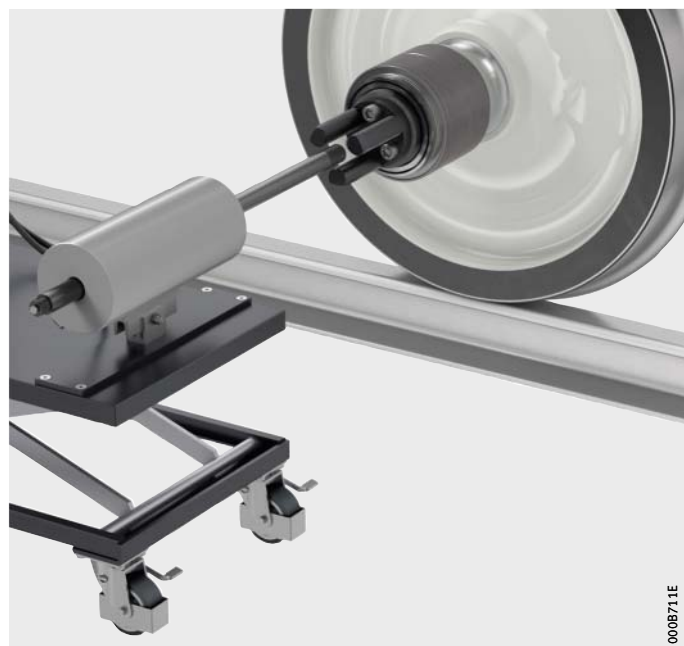
Figure 4 Inserting the spindle through the hollow piston
