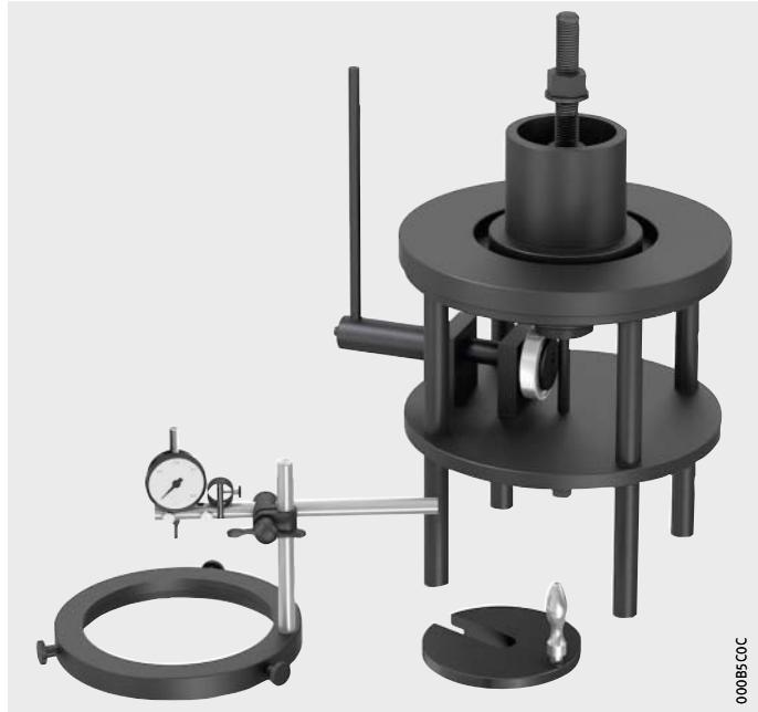
Figure 7 Fitting the centring bush
