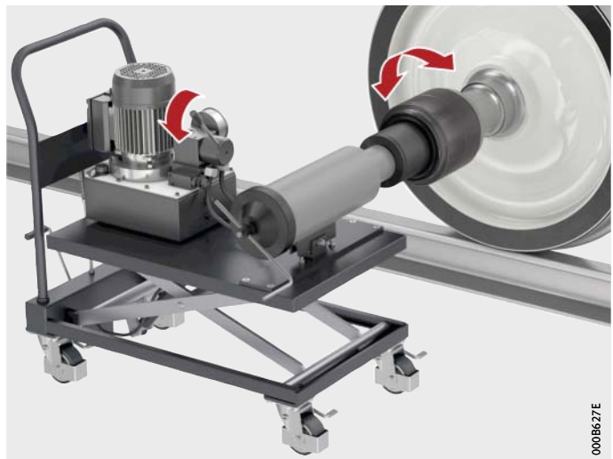
Figure 7 Pressing the bearing unit into place
