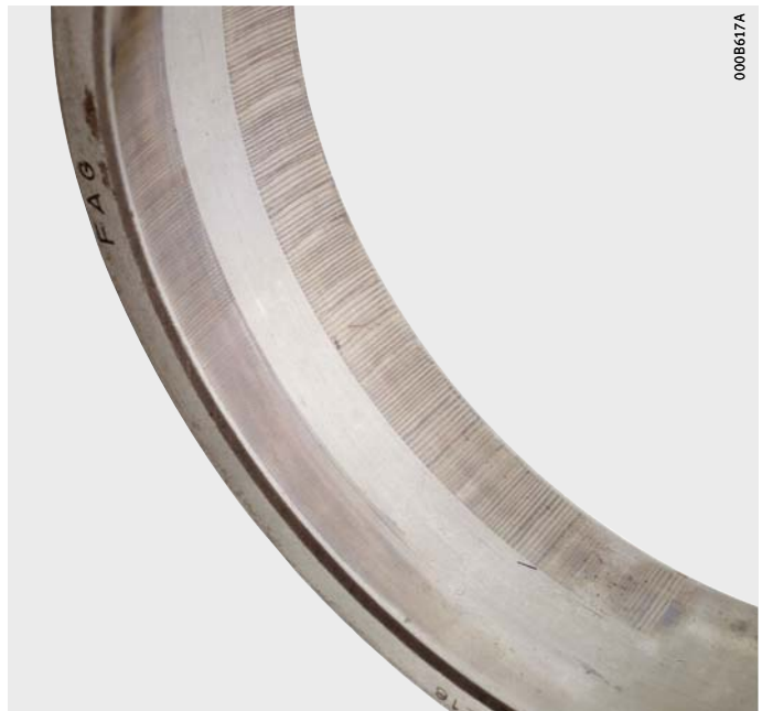
Figure 5 Current passage damage
