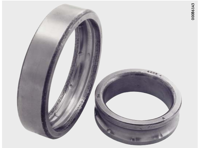
Figure 2 Rolling element indentations (brinelling)
