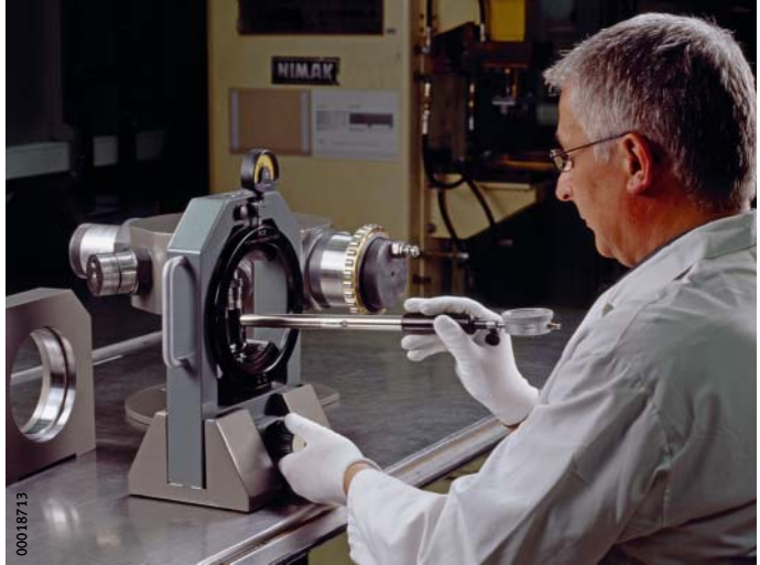
Figure 2 Transferring the raceway diameter to the enveloping circle gauge
