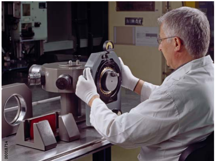
Figure 3 Positioning the enveloping circle gauge
