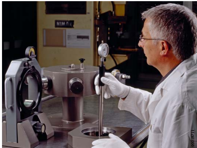
Figure 1 Raceway diameter of the outer ring
