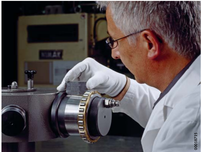
Figure 4 Measuring the distance to the shaft shoulder
